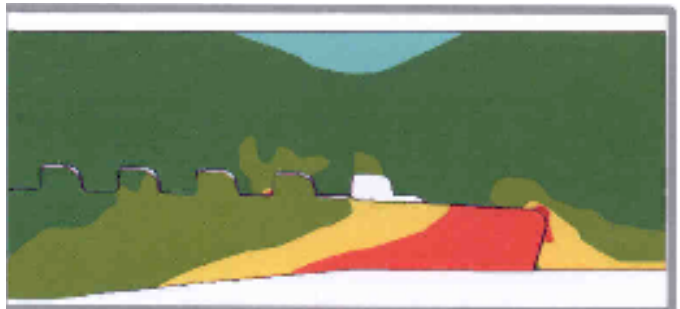
Fully Made-up with Pin Shouldering & Preloaded
