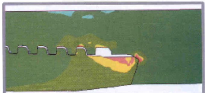
Fully Made-up with Pin Shouldering
